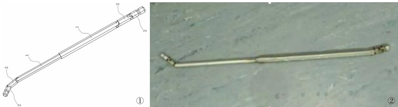
图 1 万向型螺丝刀的整体结构示意图 1:刀杆;2:刀头;3:调节件 图 2 万向型螺丝刀实物图 Fig.1 Schematic diagram of the overall structure of the universal screwdriver 1:cutter bar;2:cutter head; 3:adjuster Fig.2 Physical picture of the universal screwdriver
