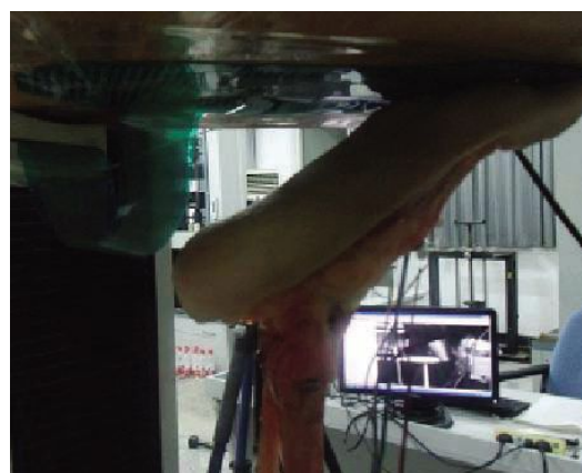
图 2 标本置于踝关节跖屈 30°位固定下加载,鞋垫式传感器仅与前足接触 Fig.2 The specimen was fixed at the 30° of ankle plantar flexion, the sole transducer could only be contacted with the forefoot
